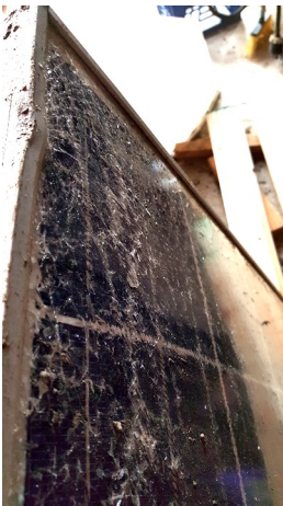
Smashed PV panel carried into shop.
